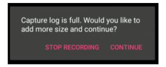
CONTINUE: the recording will resume and the new limit size will be (CurrentFileSize/1024) [in Bytes] + ConfigSizeLimit [ in Ko, specified in the configuration parameter Network.Capture.SizeLimit]
