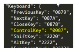
In that way, if we launch again the Keyboard Test, the F5 key has been associated with the CONTROL key
