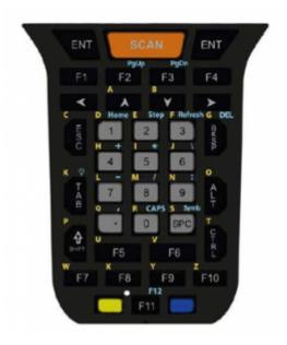
This is the Terminal Emulation Overlay for Function Numeric Keyboard (38Keys)
