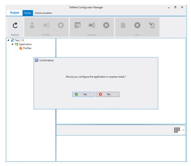
If you select Yes option, you must configure only the parameters about emulation type and the IP of the host you want to connect to. The rest of parameters will be set with the default values.
