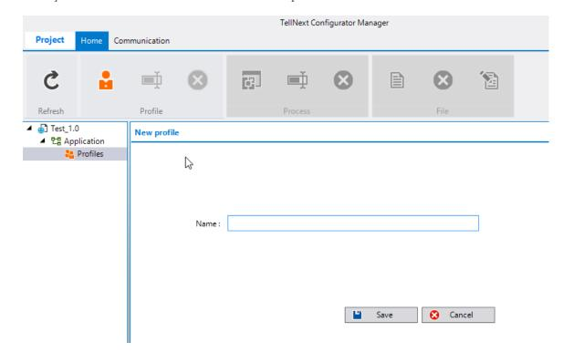
The new profile will be created (and its corresponding Processes section too) and you will have the option of review the configurated parameters through a Profile wizard or manually, with VisualJsonEditor, as we indicate in the above section.
