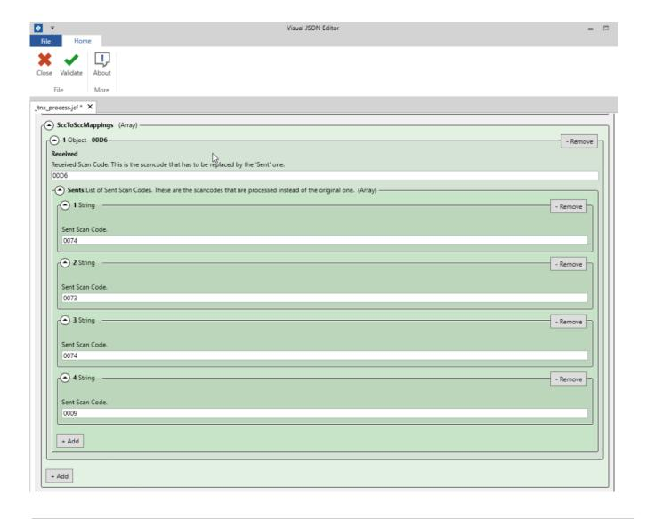
Received: write down the scan code associated to the [P1] key. The one displayed at Keyboard Test, in our case, 00D6
